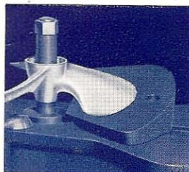
Checking a propeller on a Pitch Block
