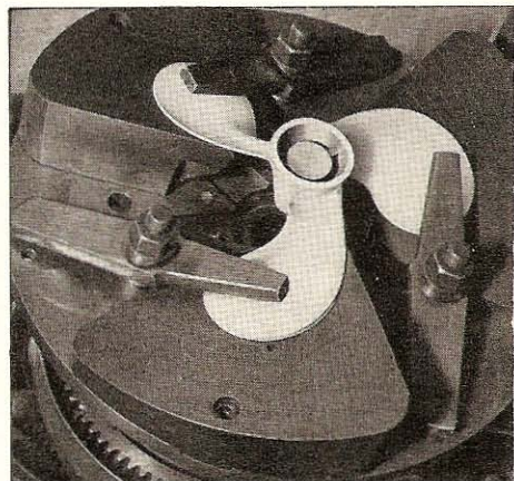
The Helical Planer, an exclusive development of Michigan Wheel Company, eliminates the human error element and carves the original patterns of Michigan Propellers and Pitch Blocks with unfailing precision and accuracy.
