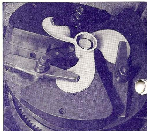
The Helical Planer, an exclusive development of Michigan Wheel Company, eliminates the human error element and carves the original patterns of Michigan Propellers and Pitch Blocks with unflinching precision and accuracy.
