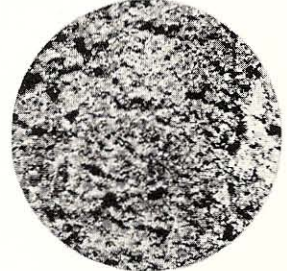
Magnified cross-sectional photo of a Michigan aluminum alloy propeller. Note the far greater density of the metal.
