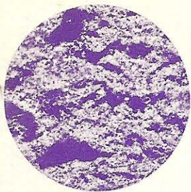
Magnified cross-sectional photo of a typical die-cast propeller. Note the porosity of the metal.
