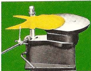
PITCH BLOCKS with true screw surfaces are used to check the accuracy of each propeller throughout the manufacturing process.
