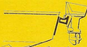
RAISED POSITION: MOTOR STORED WITHOUT CREATING "DRAG"
