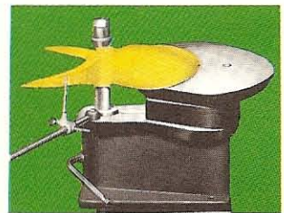
Helical Planer, a Michigan exclusive, eliminates human error - carves Michigan Prop patterns and Pitch Blocks with unflinching accuracy.
