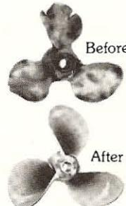
We are equipped to restore most any propeller up to eight feet in diameter to like-new condition. Field service is also assured at any of the factory-equipped Service Stations located throughout the U.S., Canada and overseas. All factory repairs are done by highly skilled workmen. Welding is handled by certified welders. Pitching or alteration work, balancing and finishing are done by leaders in their fields. Even very badly damaged propellers can usually be restored to like-new condition.
