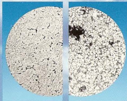
The tighter grain and compact structure of the Michigan Wheel prop on the left make it nearly twice as strong and less susceptible to damage than the ordinary prop on the right.
