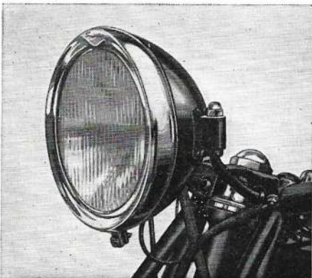
New larger headlight with chromium plated embossed rim, giving 300 per cent greater lighting capacity.
