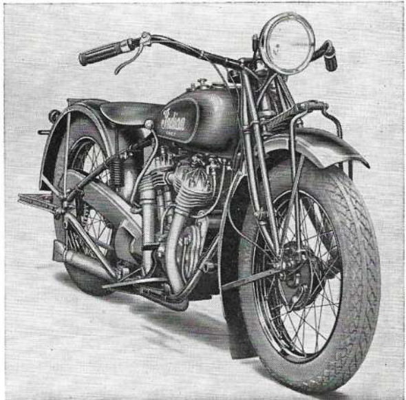
Pleasing lines of the new Chief 74 with the cast aluminum alloy saddle tanks and new low frame and saddle position. Half-a-gallon more gas in the tank, too.
