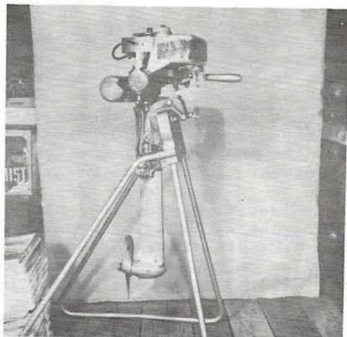
1930 EVINRUDE FOLD LITE TWIN LOWER UNIT FOLDS UP INTO RECESS OF DIVIDED MUFFLER FOR EASE OF CARRYING AND STORAGE.
