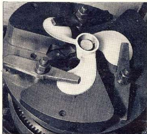
Boring a propeller by the Pitch Block Method
