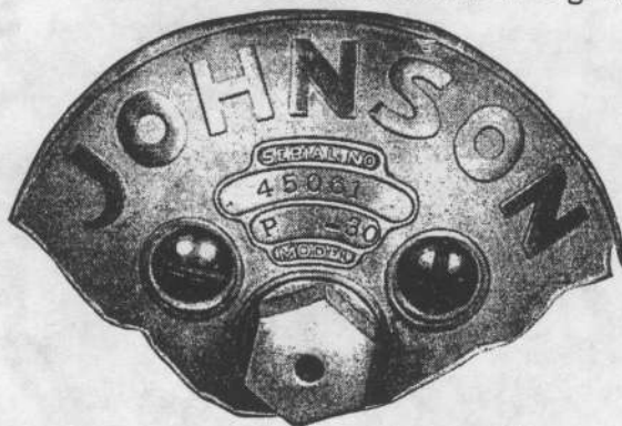
Fig. 3. Name plate, showing motor serial number
