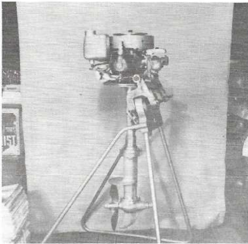
1932 MUNCIE (NEPTUNE) TWIN. MOTOR MOUNTS SOLID ON BOAT, DRIVE SHAFT HOUSING AND LOWER UNIT ROTATES 360 DEGREES. A TILLER CORD CIRCLES THE BOAT AND THE WHEEL UNDER THE MUFFLER FOR STEERING.
