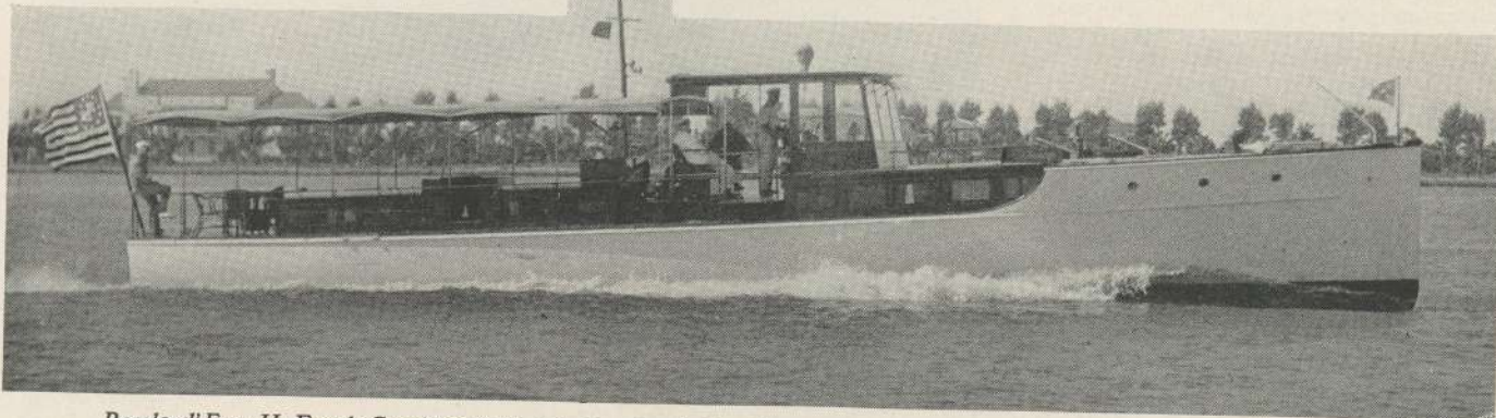
Poule d'Eau II , Frank Goodyear's 21-mile Lawley-designed 68-footer, powered with two 6-cylinder Sterling Dolphins.
