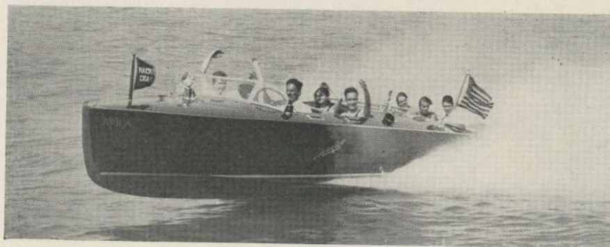
The 30-foot Hackercraft is an 11-passenger speed boat powered with the new Kermath "200." Speeds up to 43 m.p.h. are obtained.
