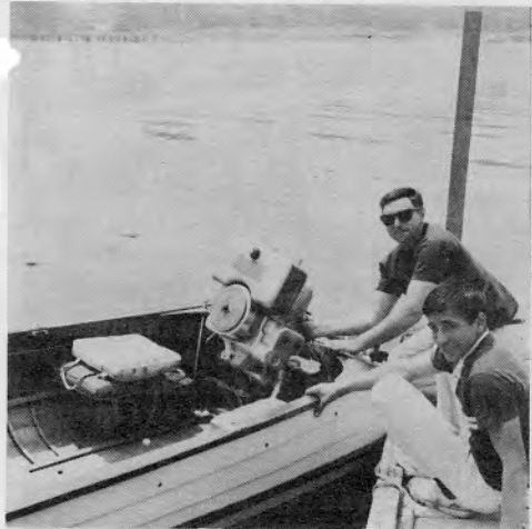
Sal (in sunglasses) and Vince Lentine of Flemington, New Jersey and Sal's 1938 Evinrude Speedifour. It ran beautifully but not for long-clogged cooling system.
