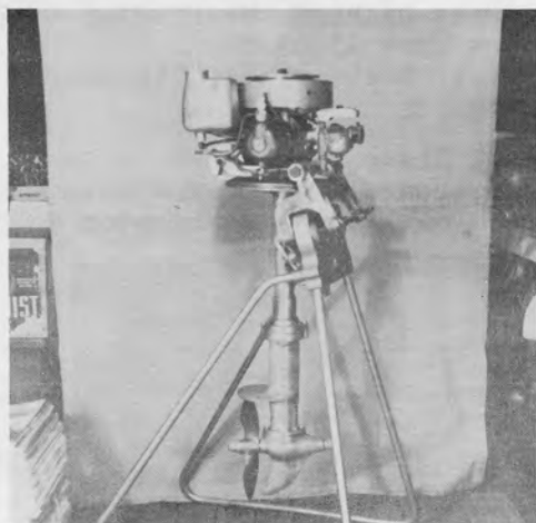
1932 MUNCIE (NEPTUNE) TWIN. MOTOR MOUNTS SOLID ON BOAT, DRIVE SHAFT HOUSING AND LOWER UNIT ROTATES 360 DEGREES. A TILLER CORD CIRCLES THE BOAT AND THE WHEEL UNDER THE MUFFLER FOR STEERING.
