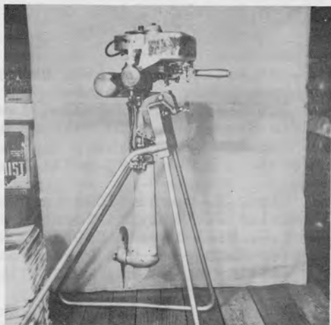
1930 EVINRUDE FOLD LITE TWIN LOWER UNIT FOLDS UP INTO RECESS OF DIVIDED MUFFLER FOR EASE OF CARRYING AND STORAGE.
