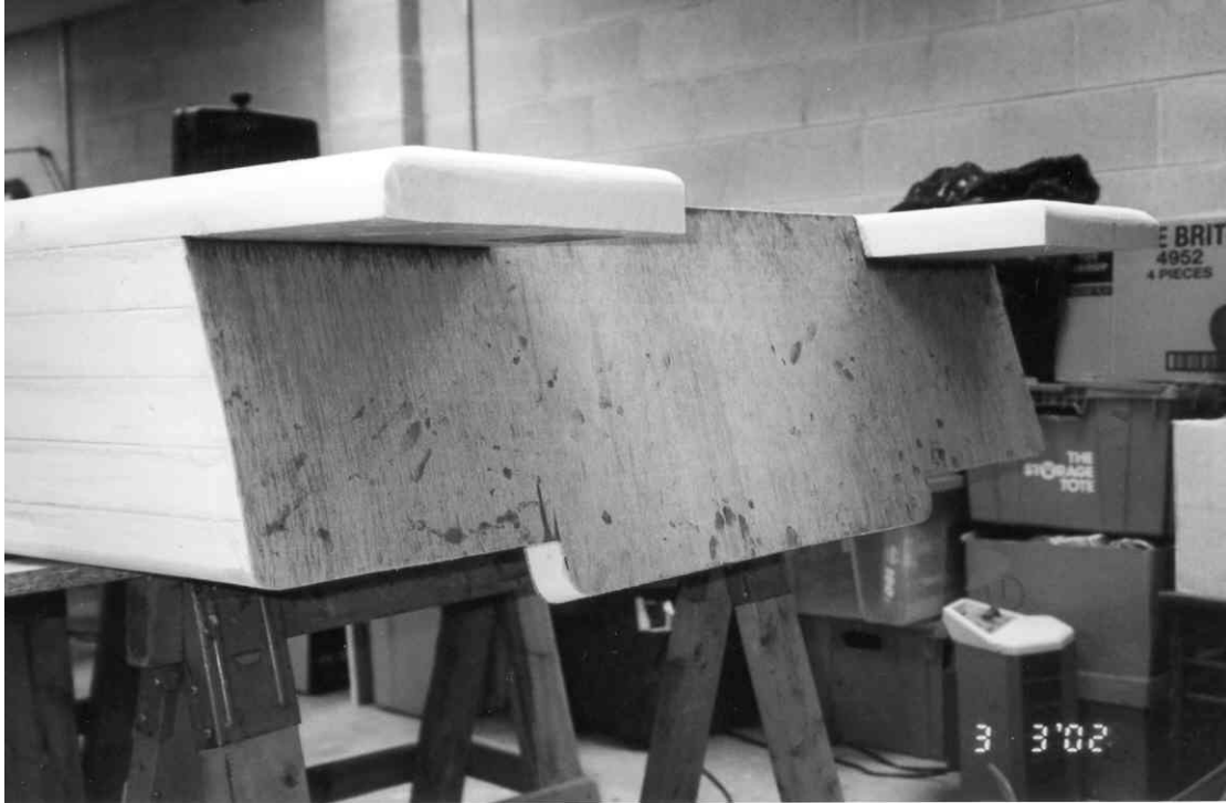
View of transom after lamination of cloth and plywood; note bottoms of afterplanes.
