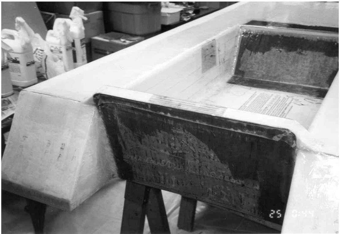
View after addition of afterplanes, fiberglass tape over top of transom, dashboard, and throttle-mount.
