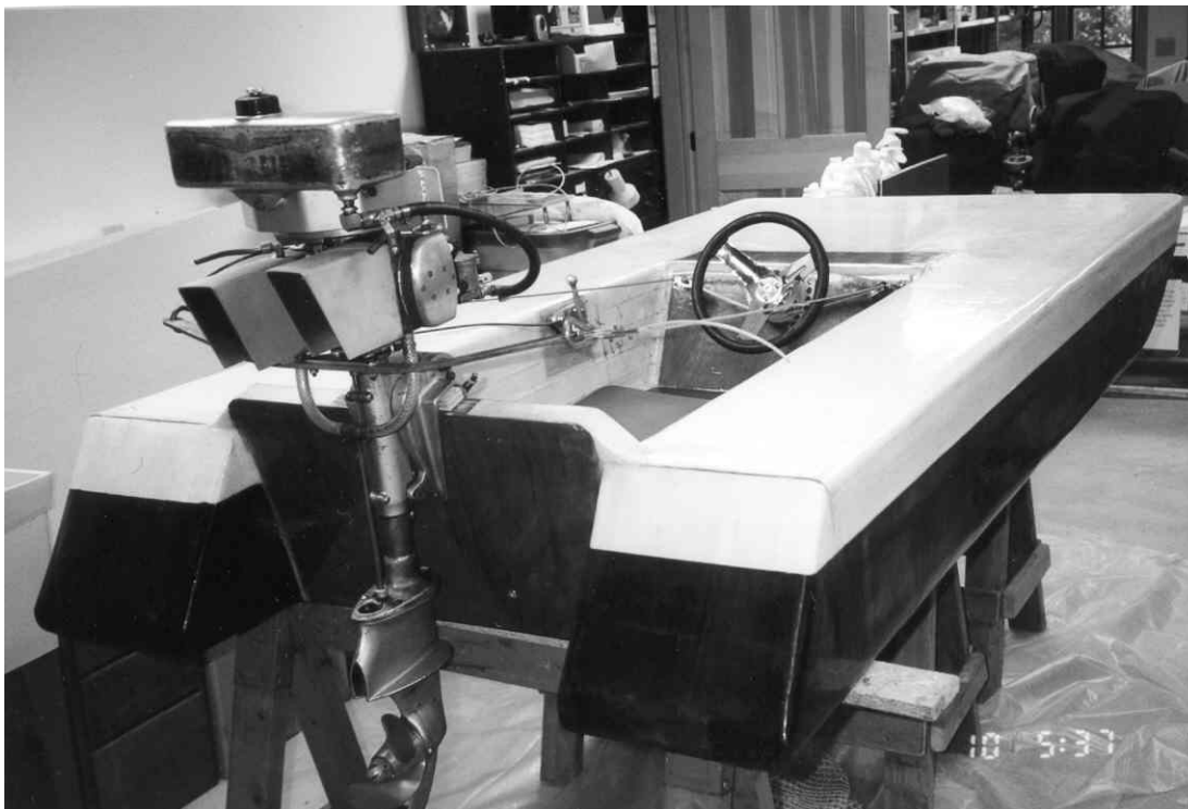
View showing all hardware installed (except for torque thrust socket) and modified Zephyr motor mounted.
