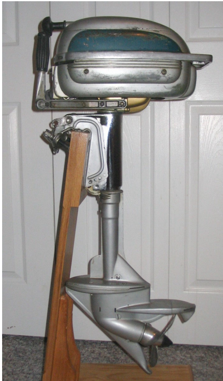
Model 4425 Evinrude Sportsman, purchased used by Stan Scratch in the early 1950's for $25. Serial number of 50556 dates this as a 1949 model. The tank decals disappeared long ago, but it still runs just as well without them.
