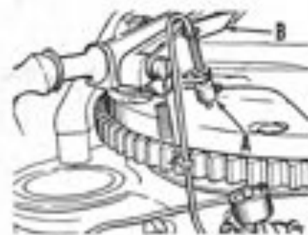
Fig. 32—To adjust the starter latch, first set speed control grip at the fast speed recommended for starting, loosen stop collar (A) and adjust latch (B) until it just clears starter pulley lugs.
