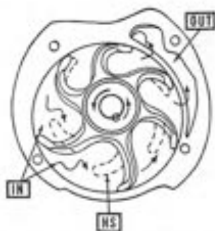
Fig. 353—Schematic view of the rubber impeller type water pump used on all models. Impeller mounts on lower unit drive shaft and rotates in upper pump housing. At slow speeds impeller blades follow the outline of housing. Water is drawn into pump (IN) as area between blades increases, and is forced into power head (OUT) as area narrows. At high speeds, blades remain curved as shown by broken lines (HS) and pump operates by centrifugal action.
