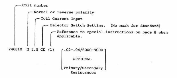
Primary and secondary coil resistances, which can be measured with the Lo and Hi Resistance functions of the ST-75, are often available with the engine manufacturer's service literature. Some of these readings are also furnished in the following specifications, immediately following the specs for coil power test, as shown above, marked "Optional".
