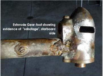
butchery was that possibly the setscrew for the prop-shaft pinion had become seized or broken, and the window had to be cut to facilitate removal. A tin patch was laid over the hole and soldered in place in an attempt to seal up the hole. I don't think it was a factory-authorized fix-it job, but it wasn't something to give up on. The decision was made that the parts were salvageable, so the task was undertaken to attempt to correct the previous "repairs".
