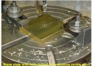
center point was located and a ¼ inch hole drilled to allow me to indicate the plate on the rotary table, then I could accurately machine the outside & inside diameters, as well as the outer profile for the mounting lug that protrudes from the front end of the muffler cap. This same method could be used to make the bottom cap, which is actually a simpler part to mill; its just a round cap, it doesn't have the mounting lug sticking out the front of it like the top one does.
