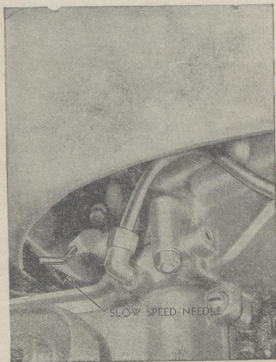
Fig. 14. Showing Location of Slow Speed Needle on Model TSL.
