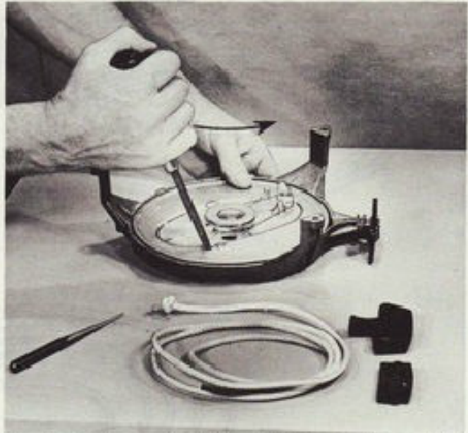
Winding Starter spring to full tight. A screwdriver blade tapered down and bent over at the tip as shown below will do nicely for this operation. Remove burrs and sharp edges from the tool to prevent scuffing of the Starter plate.
