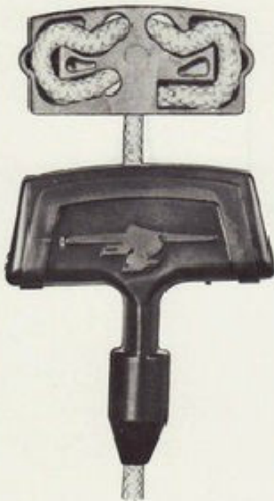
Some starter plate covers are provided with a hole into which a punch may be inserted to hold the plate in desired position for "threading" of the Cord.
