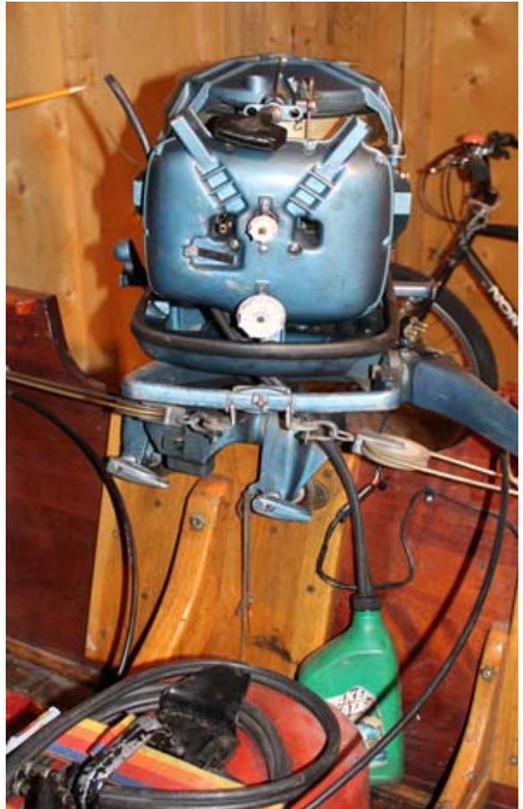
My experience has been, if I operate for extended periods at less than cruising speed, I collect almost a litre of fuel and oil per 20 litre tank of fuel burned. This I just simply pour back into the tank when I refill it. However, if I run predominately at cruising speed (well, being honest, wide open throttle) I'll collect only about a cup per tank.
