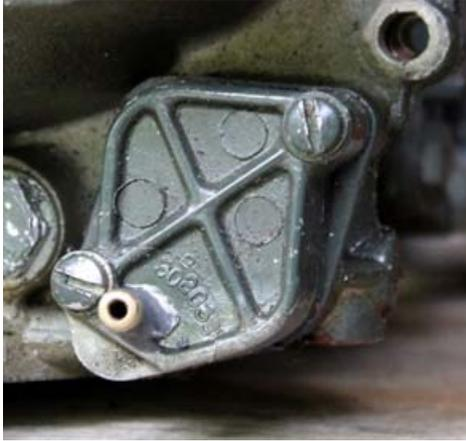
Reinstall the cover plate, connect a hose to the fitting and run it to an approved gasoline container. At least that's what **you** should do. As you can see, I ran mine to an old oil bottle.
