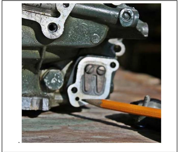
Remove this cover plate and you will see the backside of two check valves and, at the lowest point, a small hole. With every power stroke, any fuel/oil pooled in the cylinder's crankcase is blown through these check valves and out the bleed hole in the block to the exhaust leg.
