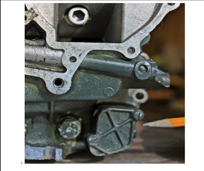
On the 50's and 60's era 25 hp and up OMC engines, there is a small parallelogram shaped cover plate at the lower front of the engine. It's accessible with the lower engine pan on, but difficult to see, so for the purposes of photos, I've used a parts-donor 33 hp block.
