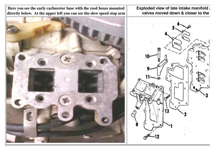
**Reed Valve Boxes**: As said above, the reed valves in these 9.5 motors were two different types. The early version used a set of reeds mounted in removable boxes that sat under the carburetor base and accessible only from that location. This adapter plate is held in place by two opposing Phillips head screws, which over time could become hard to remove without the aid of an impact driver as seen in the photo above. In this photo the reed box screws were already removed.
