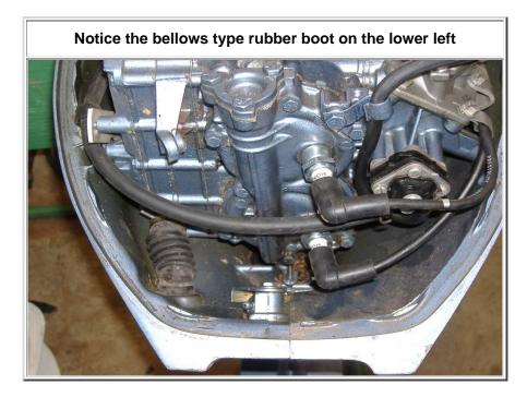
housing. A tip to install it, is to lubricate it with some soapy water. It goes into a hole slightly smaller than the outer end of the boot, which snaps over the outer part of the hole, holding the boot in place.
