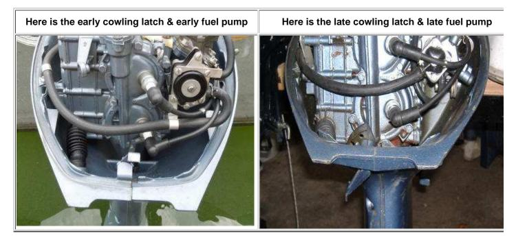
*Lower Cover*: These motors utilized a split lower cover that surrounded the exhaust housing. This feature compounds repairs where a simple part may need to be replaced, but the whole cover needs to be removed to access it.
