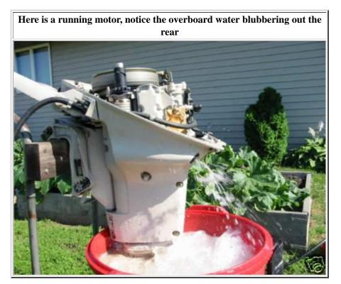
Water mix will only spray out that hole when the thermostat is open. So until the motor warms up, it should be dry for possibly the first minute or so when started cold. In the photo below, you will see the thermostat cover plate center top of the photo held in by the 3 bolts.
