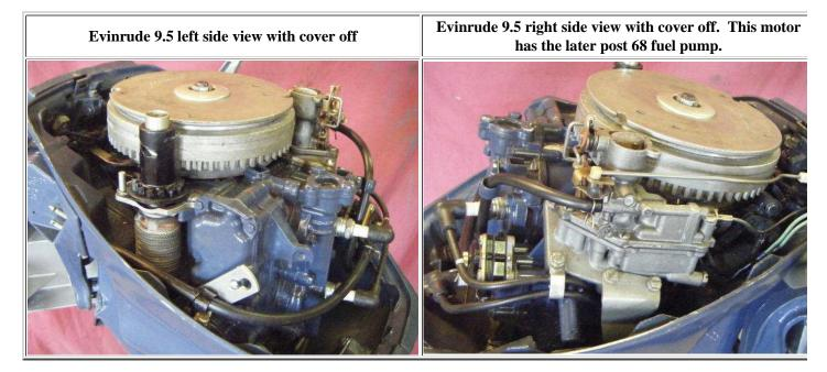
**Recommended Spark Plugs**: The recommended spark plug is a Champion J4C, however with a well used motor most old time mechanics would recommend a hotter plug, like the J6C especially if you do a lot of trolling. Or if you opt for the NGK brand, go for BR6S-8. These plugs use the 3/8" reach thread length, so do not try to use the 1/2" reach ones off the 9.9hp as the electrodes will become smashed by the top of the piston.
