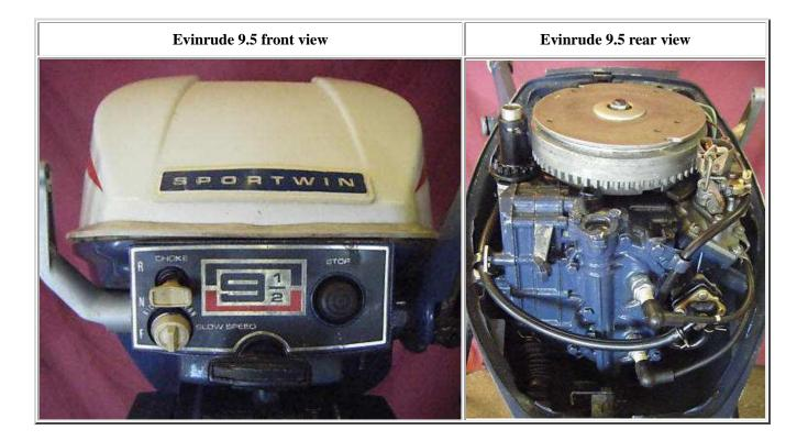
**Upper Cowling**: There were 2 different type of cowling latches, a twist lock that was made only in '64 and '65. They moved the release lever into the lower cowl in '66, but pretty much all the other parts on that are interchangeable.
