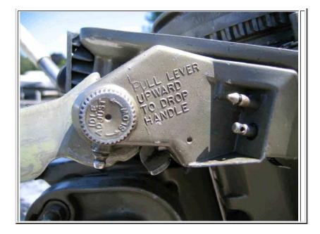
*Tilt Lock:* When the engine is tilted up, it is held in place by the large rod (on the right when looking at the engine from the front side). In addition, there is a ratchet mechanism to the left (visible on the attached LH photo below) which prevents the engine being lowered by it's own weight.
