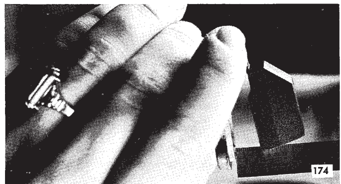
FIGURE 15 — CHECKING FLOAT LEVEL
