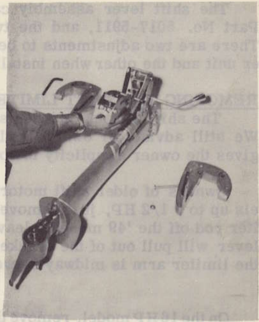
Replacing tilt arm assembly.
