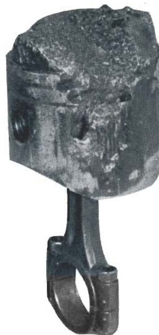
A burned piston is the result of incorrect tuning adjustments or a clogged cooling system. Always make tuning adjustments accurately.
