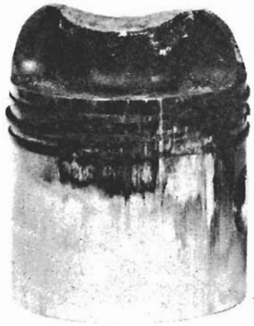
Using the wrong oils or an incorrect mixture of oil and gasoline can result in piston scoring. Follow the manufacturer's instructions to protect your outboard motor.
