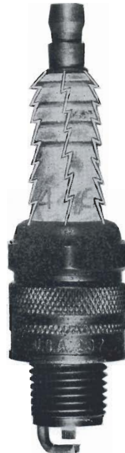
When the dirty insulator of a spark plug gets wet, flash-over occurs, and the cylinder misfires.
