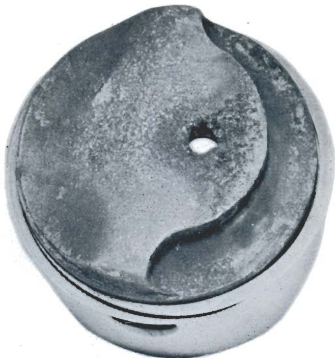
This hole in the piston crown is the result of runaway surface ignition. It can be caused by a lean carburetor mixture or the ignition timing's being too far advanced.
