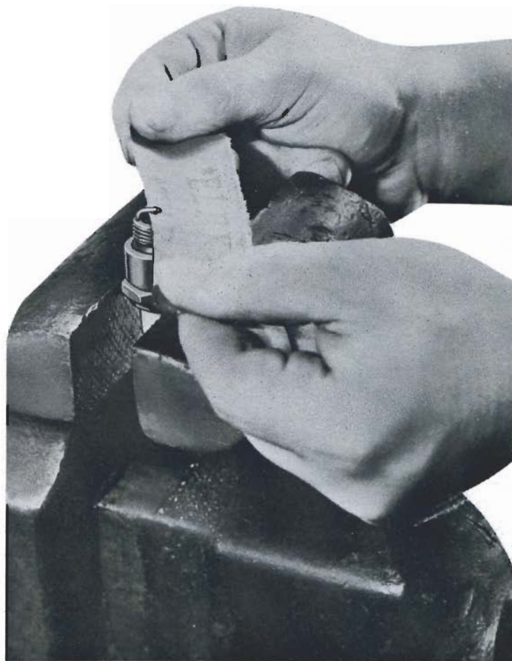
One of the most important spark plug service procedures is to file the electrodes to remove the corrosion. This mechanic is passing a piece of emery cloth between the electrodes to clean the metal.
