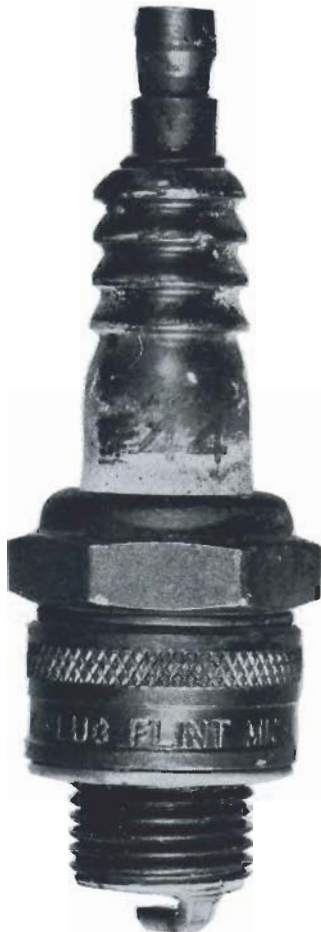
The spark plug insulator should be cleaned of all foreign matter, because this could become a leakage path for the high-tension voltage.
