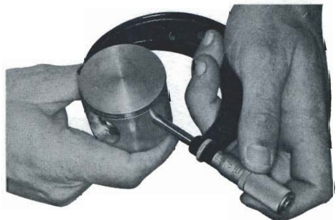
Measure the diameter of the piston just below the ring lands to determine the amount of wear.
