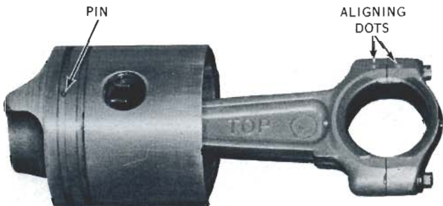
The alignment pin for the top ring groove must be on the same side as the aligning dots.
