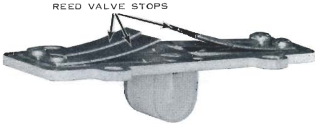
The reed-valve stops should be 1/4" above the reed valves. CAUTION: The reed valves must cover the openings in the block perfectly.
