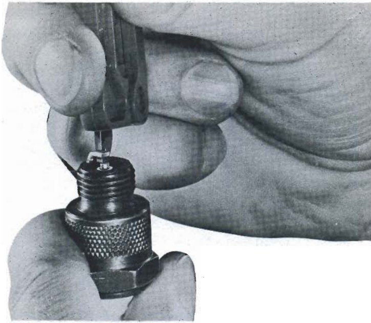
Always bend the ground electrode to adjust the gap. If you bend the center electrode, you will crack the porcelain.
