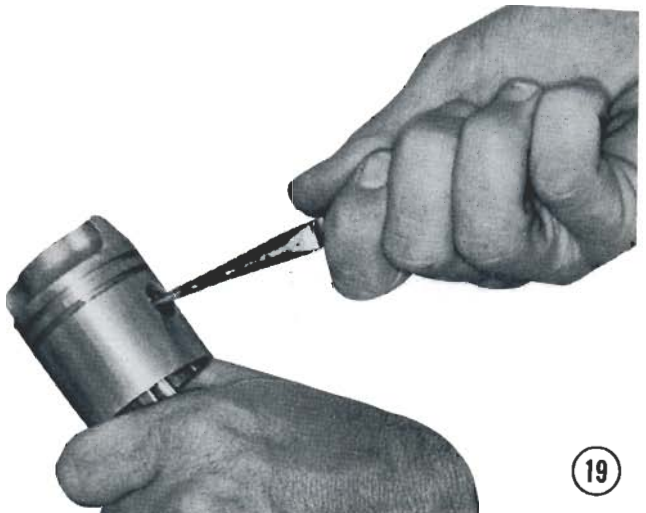
The alignment pin for the top ring groove must be on the same side as the aligning dots.
